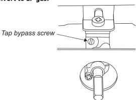
Turn the bypass screw on each control clockwise to the stop.
